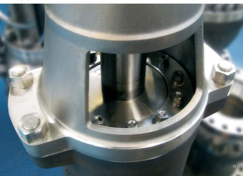
PRESSURE SEAL DESIGN (HIGH PRESSURE APPLICATIONS)
