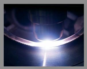
"INTERNAL WELD OVERLAY OPTIONS FOR ABRASIVE AND/OR CORROSION APPLICATIONS ARE AVAILABLE".
